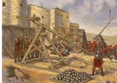
A trebuchet is a **lever**. It uses a **small force** to have a **greater effect** – a small force to throw the heavy rocks.
